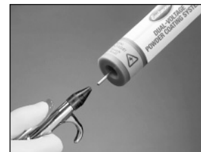
Direct air nozzle down to remove powder
