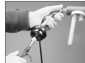
Press trigger and blow remaining powder out of the discharge tube
