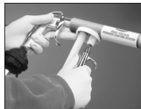
Blow remaining powder out of pick-up tube
