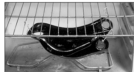
Use Stainless Steel Safety Wire (#43045) to suspend parts from rack
