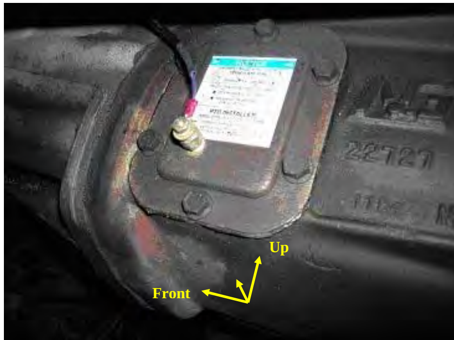
Figure 22 – Manual Transmission Temperature Sensor Location
