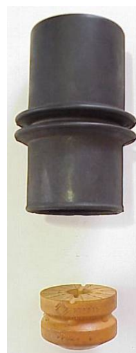
Insert Eibach Bump Stop into OE Dust Boot & install on Strut.
