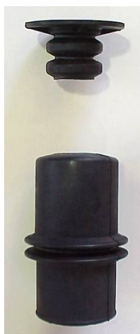
Trim Front Bump Stop away from Dust Boot as Shown
