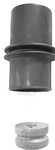
Insert Eibach Bump Stop into OE Dust Boot & install on Strut.
