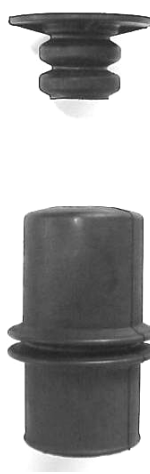
Trim Front Bump Stop away from Dust Boot as Shown
