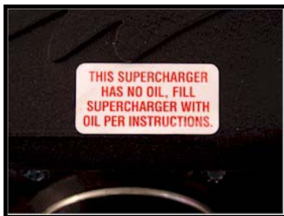
Warning label attached to Supercharger housing
