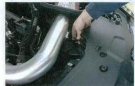
1A. Attach the factory mass air flow sensor harness connector to the mass air flow sensor. Pay close attention to the direction of the connector when installing. Push in red clip after connector has mated.
