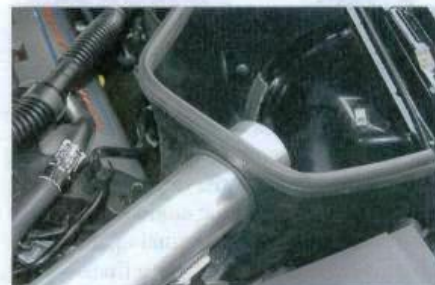
W. Guide the GMS intake tube through the air box opening. Use caution not to push out the rubber seal. A small amount of water aids in lubrication for installation.
