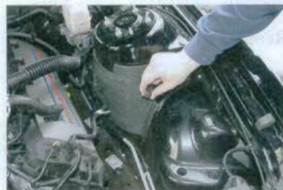
N. Remove the plastic fender grommet by pulling gently with a panel removal tool or a pair of pliers. Take extra caution not to break grommet.
