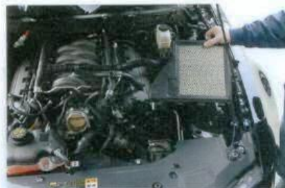
M. Pull up gently on lower air box portion and remove.
