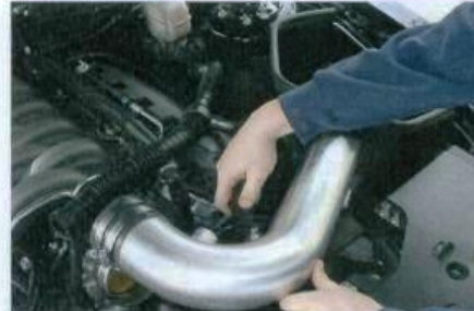
X. Re-connect the factory vent tube to the GMS intake tube, by holding back on the clip and pushing firmly until it clicks.
