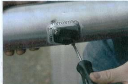
V. Secure the mass air flow sensor with the two provided 4mm bolts.
