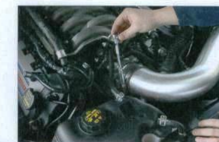
Z. Slide the GMS tube and coupler assembly onto the throttle body. Secure it with the two stainless hose clamps provided.
