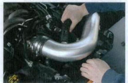
Y. Re-connect the sound tube to the GMS intake tube and secure it in place with the factory spring clamp.
