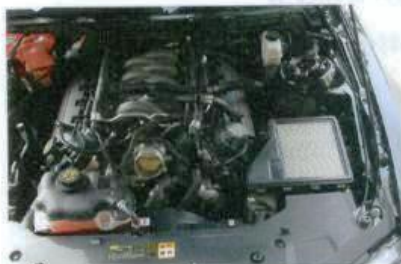
K. It is now time to lift up gently on the top of the air box and remove the entire upper assembly
