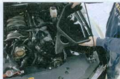
P. Gently guide and lower the GMS airbox into position. Make sure the inlet of the airbox mates with the factory air scoop.
