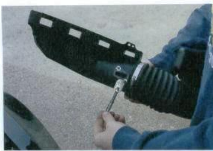
T. Remove the two Torx screws from the factory air box along with the factory mass air flow sensor.
