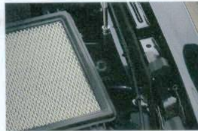
L. Remove the bottom portion of the air box by removing the secured M6 bolt.
