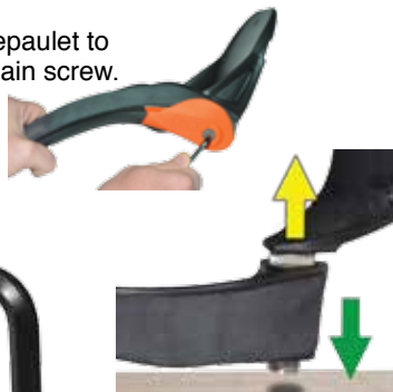
3. Strike main screw gently against firm, soft surface or strike with soft mallet to slide leg off splines.
