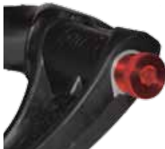
2. Thread leg removal tool slowly into leg.
