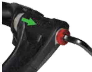
3. Tighten tool to slide leg off splines.
