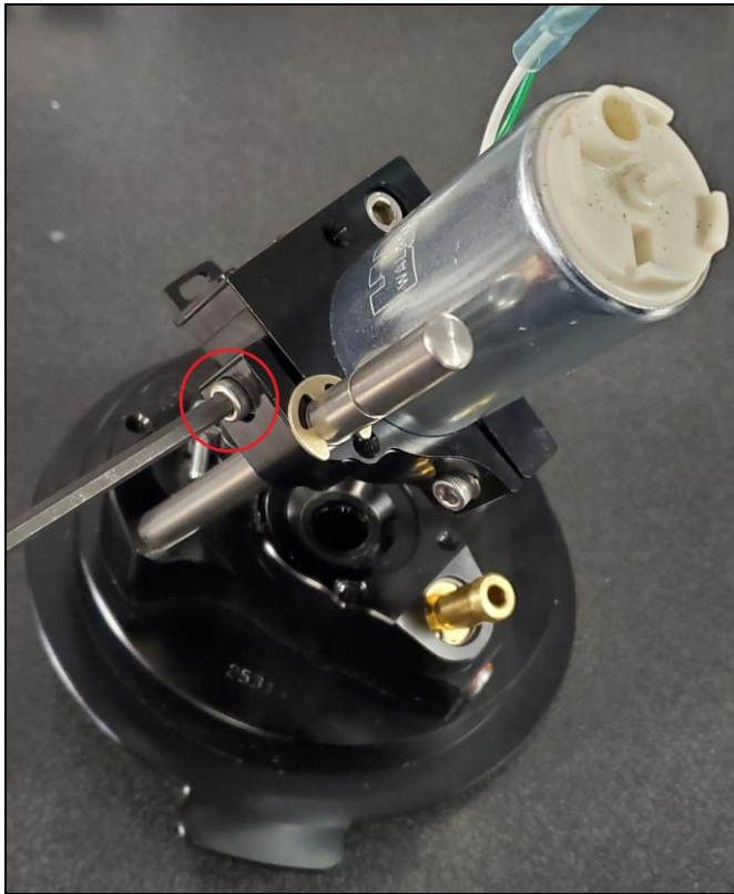
Figure 1 - Pump clamp retaining screw
