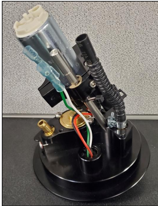
Figure 4 – Final assembly – Return tube zip tied to guide rod.
