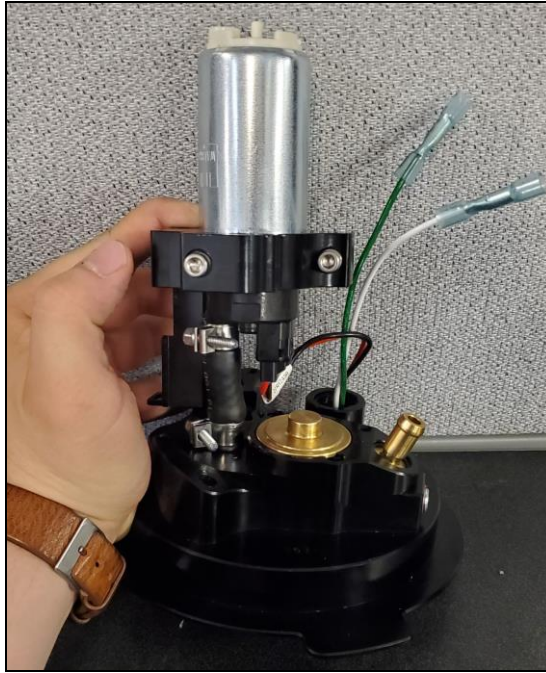
Figure 3 – Pump guide rods removed, pump moved, and regulator plug installed
