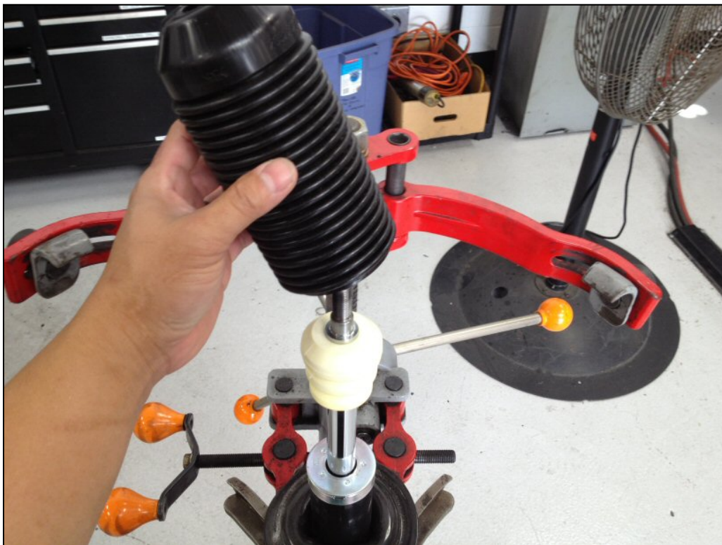
11F. Cut the OE bump stop as shown in the picture.
