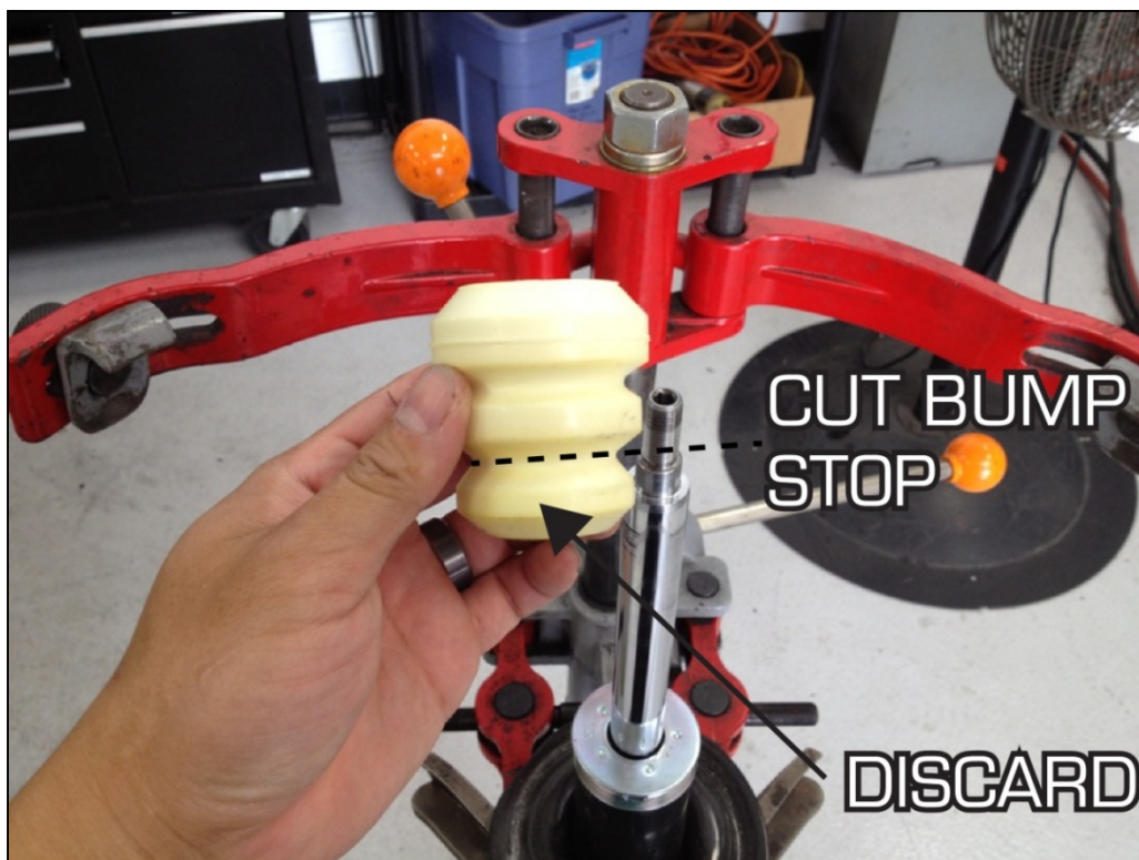
11F. Cut the OE bump stop as shown in the picture.
