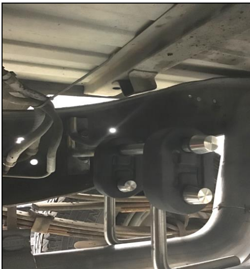
Figure 1 After muffler hanger rod attachment to frame
