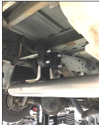
Figure 2 Rear tailpipe hanger to frame
