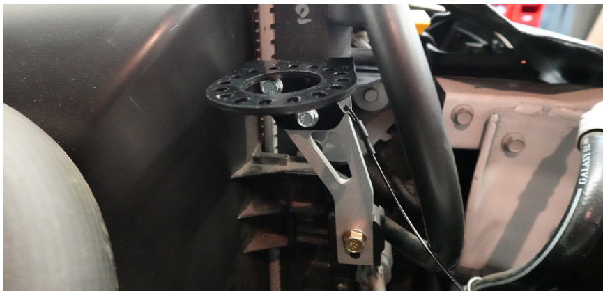
Figure 9 - Installed Catch Can Bracket
