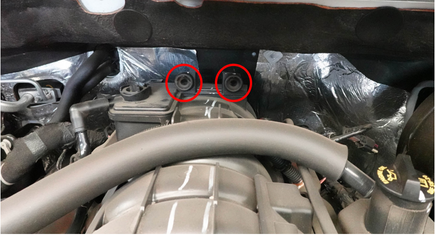
Figure 3 - Intake Manifold Engine Cover Post Holes
