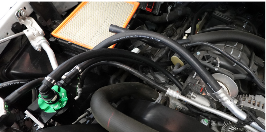
Figure 12 - Installed Catch Can Lines
