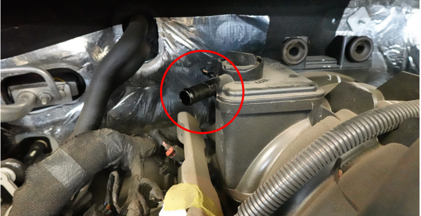
Figure 5 - PCV Crankcase Outlet
