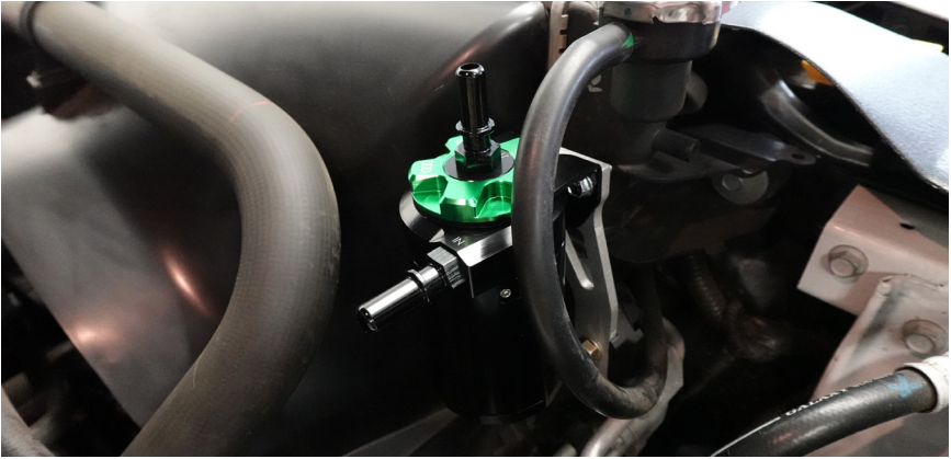
Figure 11 - Installed Catch Can
