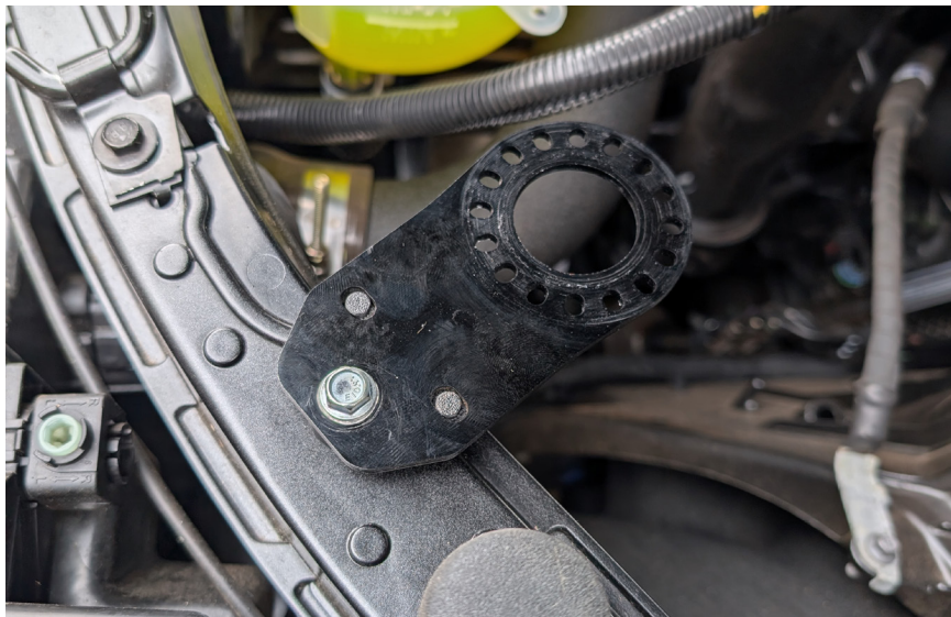
Figure 6 - Mounted Bracket on Core Support (2025+)
