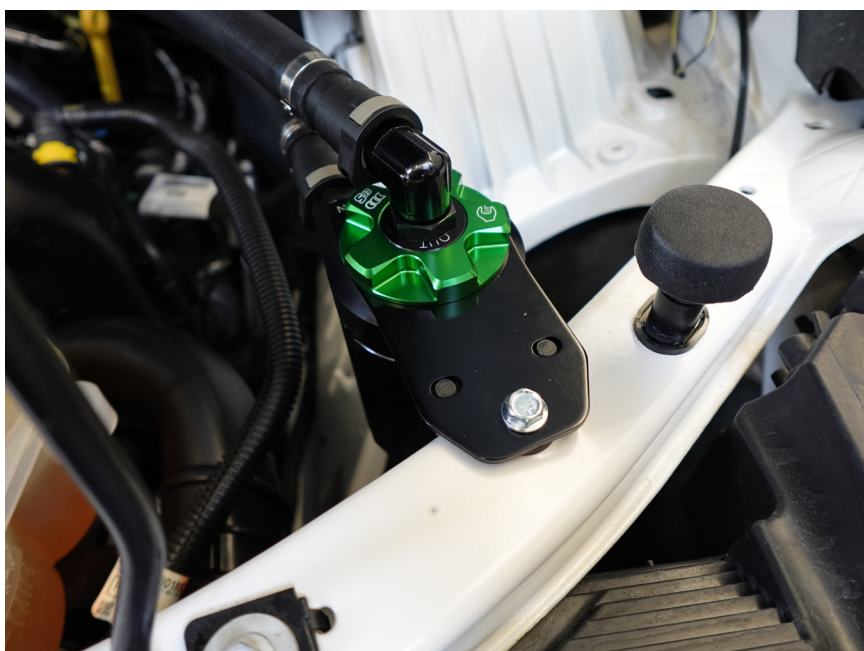
Figure 8 - OUT Adapter Fitting Placement
