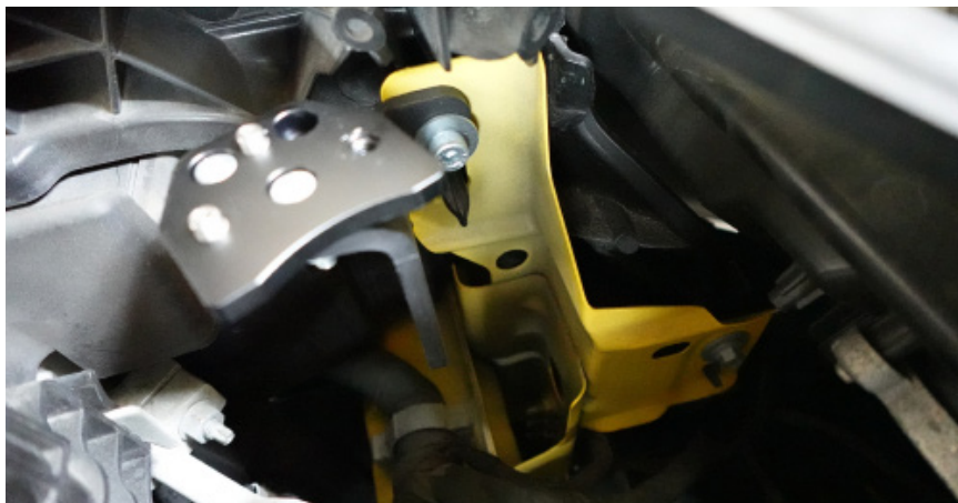
Figure 6 - Catch Can Adapter Bracket Mounted
