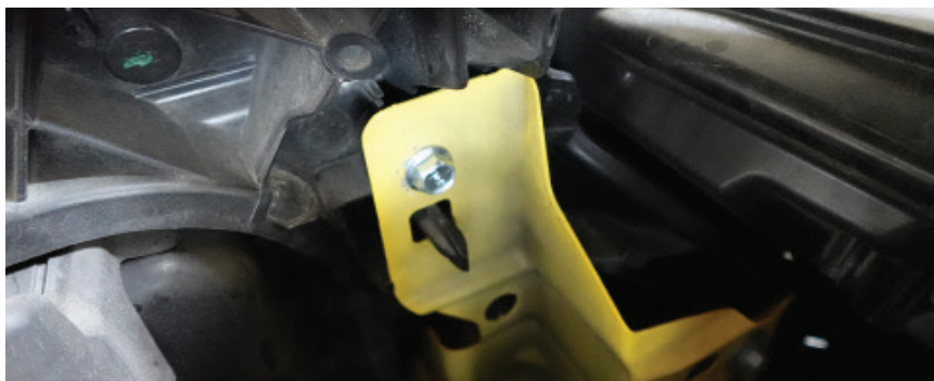
Figure 5 - Adapter Bracket Mounting Point
