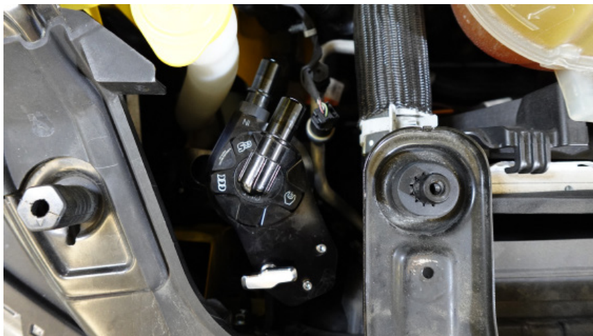
Figure 9 - Catch Can Installed on Adapter Bracket
