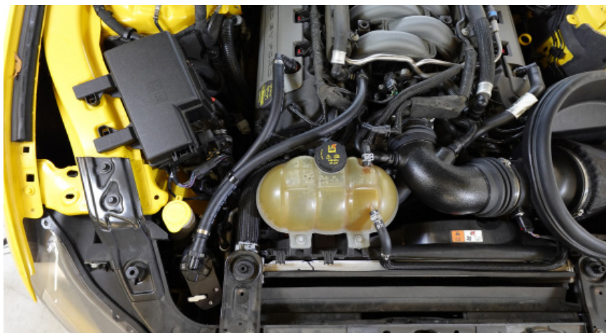
Figure 10 - Catch Can Hoses and Hose Separator Installed
