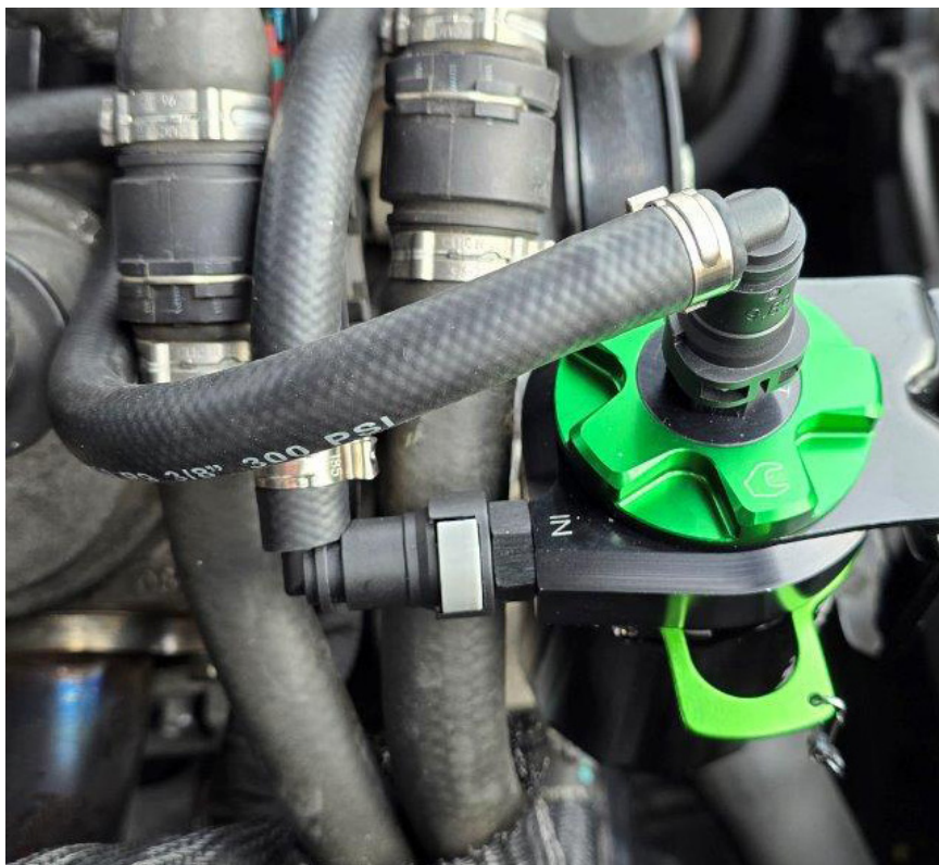
Figure 6 - Final Hose Routing
