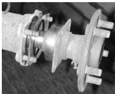
Installation of Spacer Plate.
