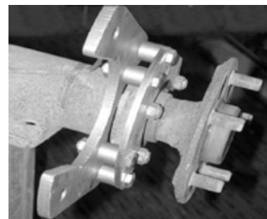
Installation of caliper bracket.
