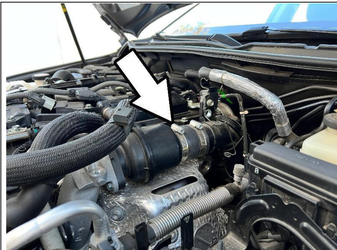
9. Loosen the hose clamp securing the intercooler hose to the turbo resonator.
