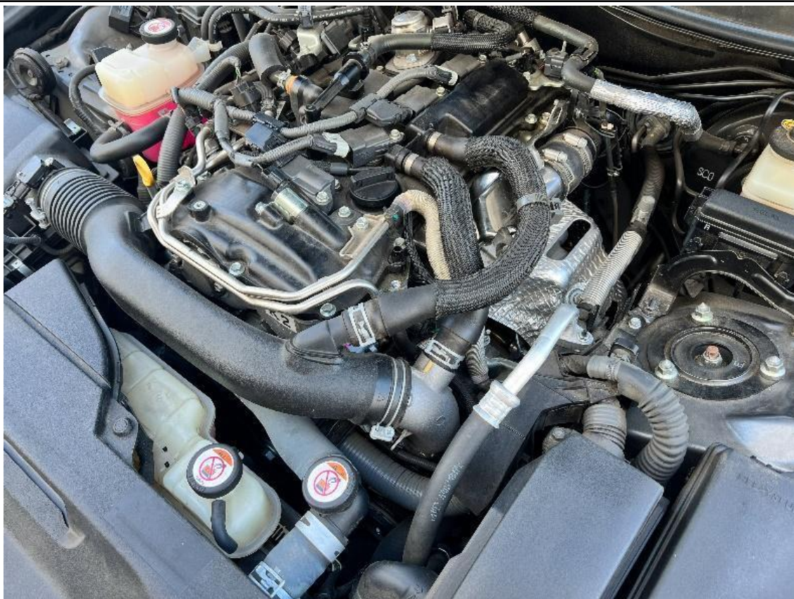
18. Reinstall the heat shield back into the vehicle and reconnect the breather hoses. Clip the vacuum hose back onto the turbo outlet elbow.
