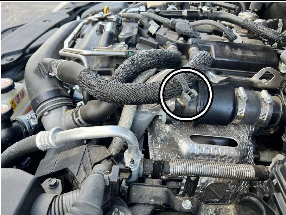
3. Disconnect the retaining clip securing the breather hose.
