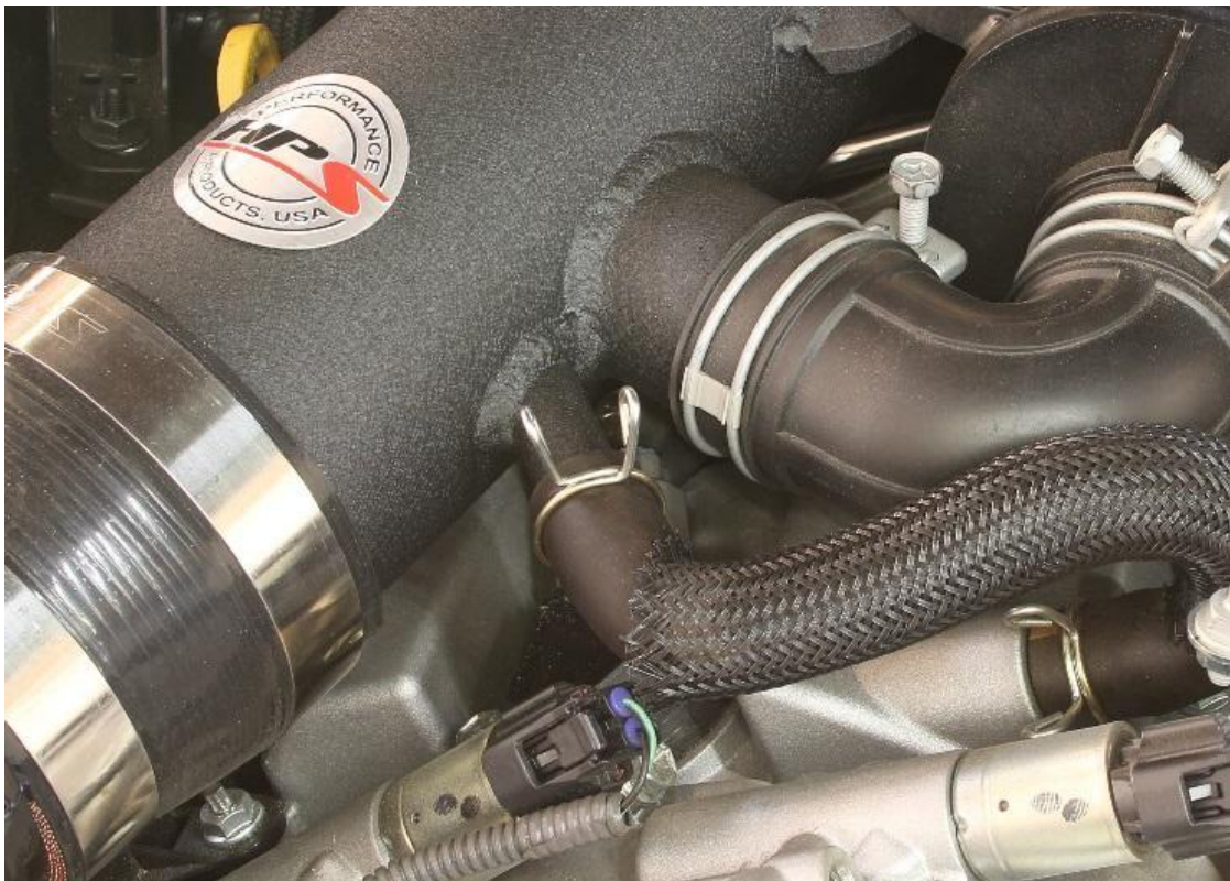
14. Connect the stock breather hose to the new intake.
