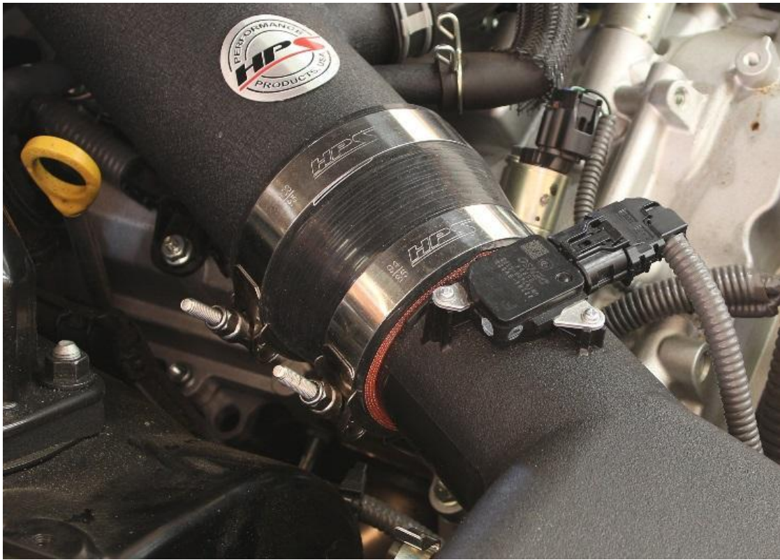
13. Insert the other end of the HPS intake pipe into the coupler at the air box.
