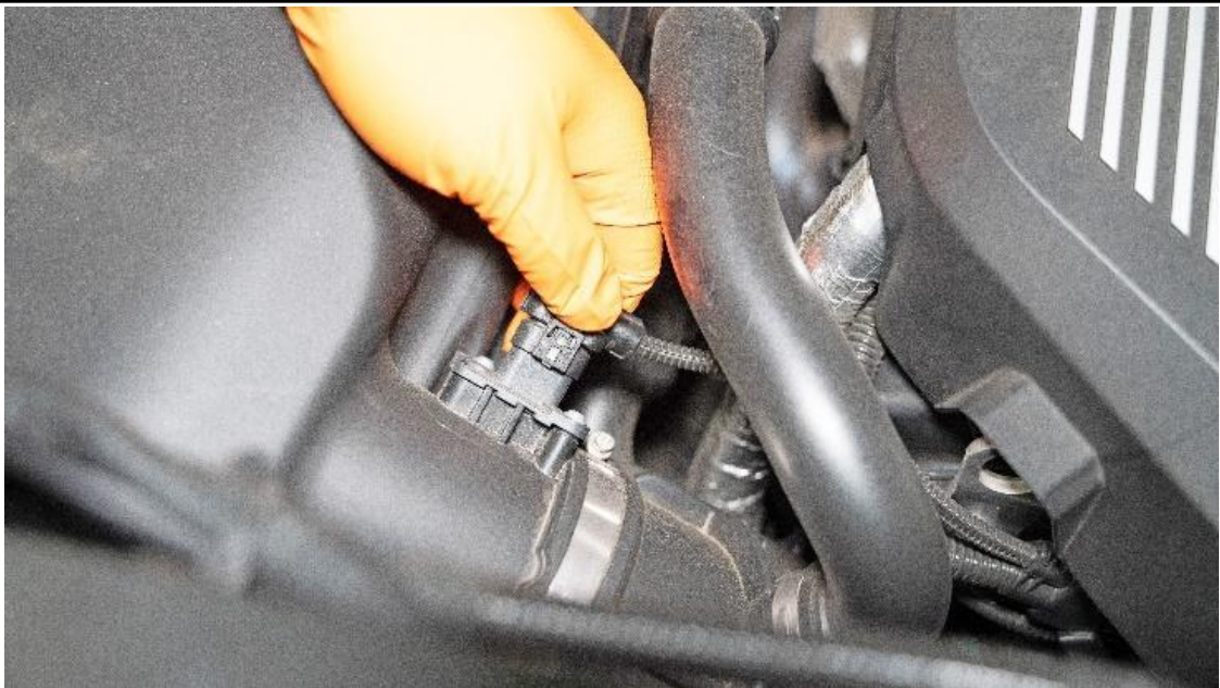
3. Disconnect the mass air flow sensor electrical connector.
