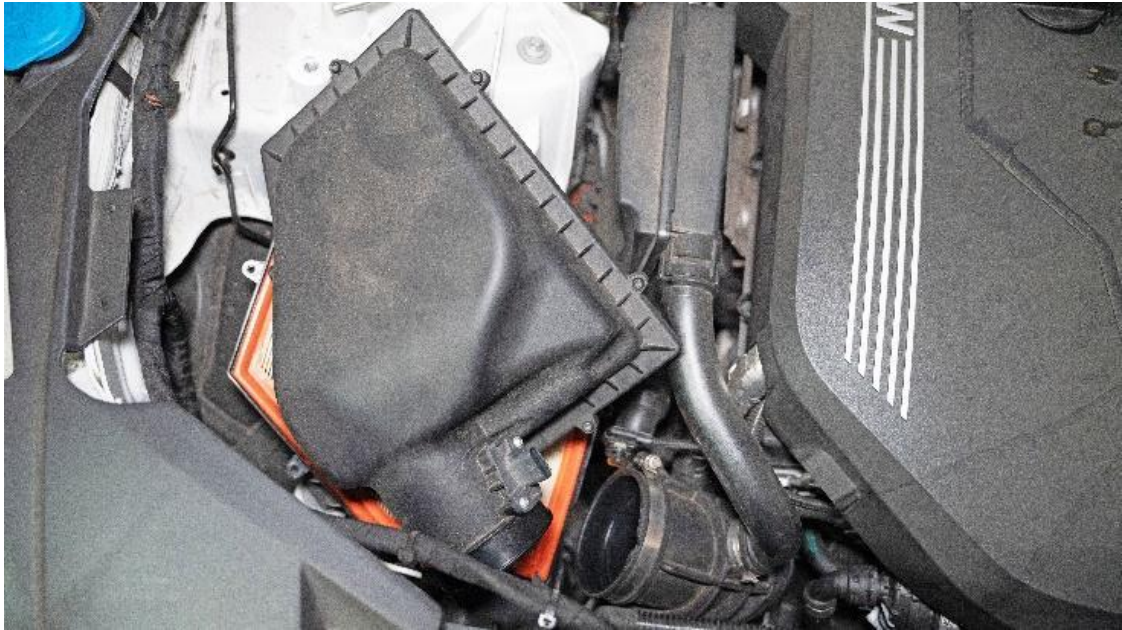
6. Disconnect the upper air box from the intake hose and remove it from the vehicle.
