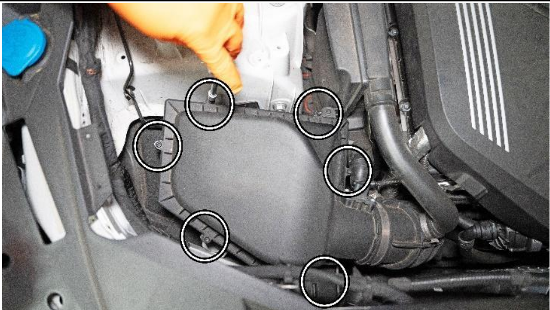
4. Loosen the six bolts securing the upper air box using a T25 Torx bit.
