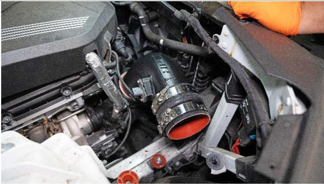
15. Slip the HPS intake into the reducer coupler at the turbo inlet.
