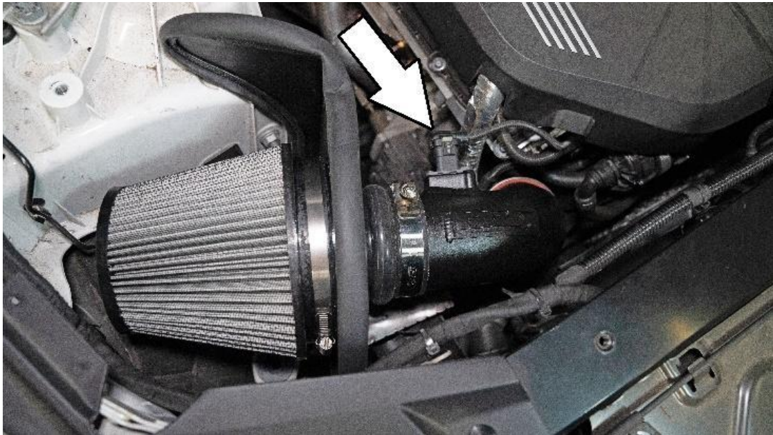
20. Secure the HPS performance air filter to the velocity stack and then reconnect the MAF sensor.
