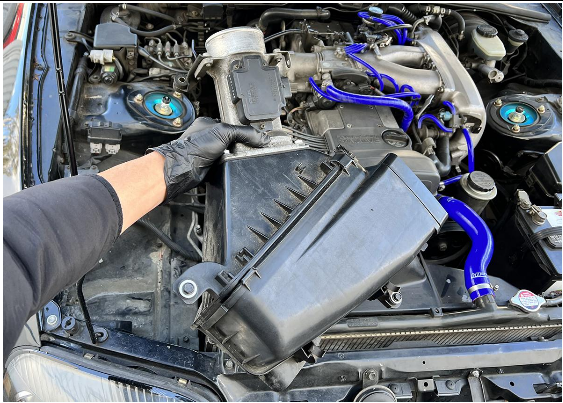
11. Remove the air box assembly from the engine bay.
