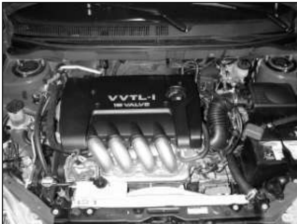
Factory air box system installed
