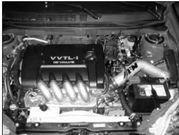
AEM® intake system installed
