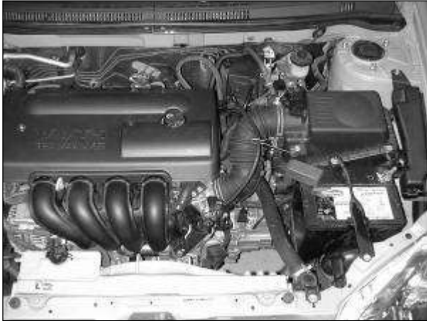
Factory air box system installed
