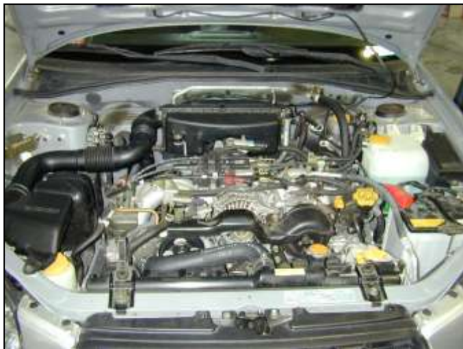
a. Factory air box system installed.
