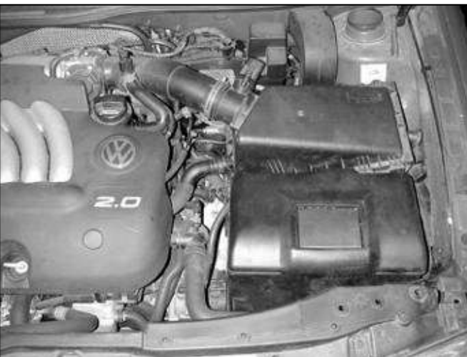
Factory airbox system installed
