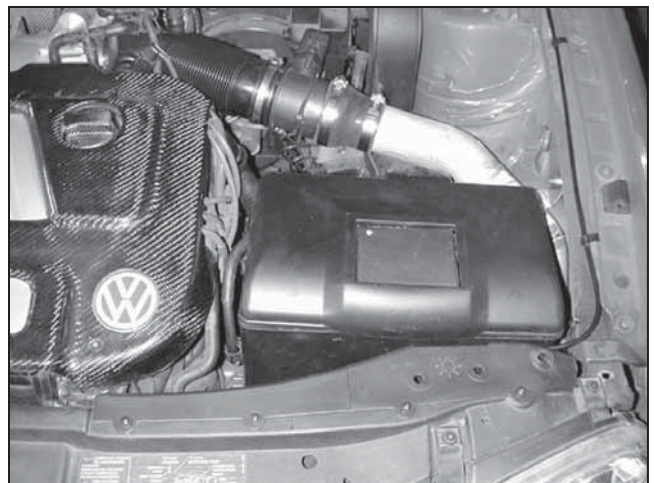
AEM® intake system installed
