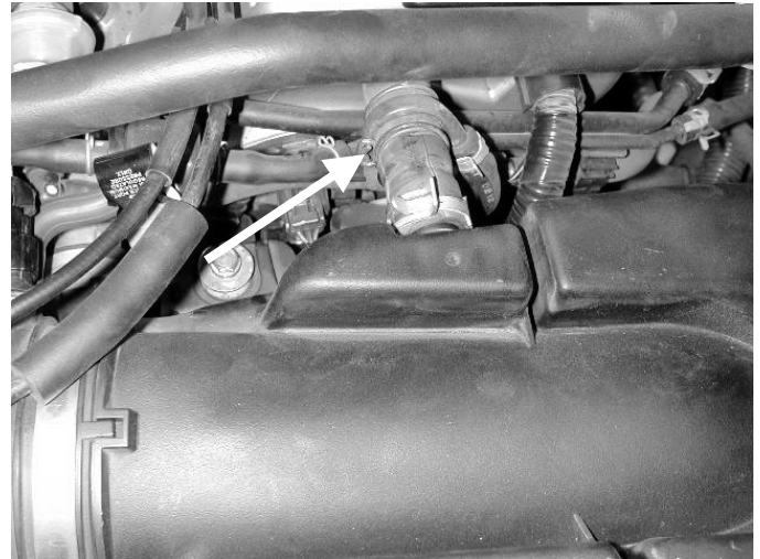
d) Pinch the clamp that secures the crankcase breather hose and pull the hose from the nipple.
