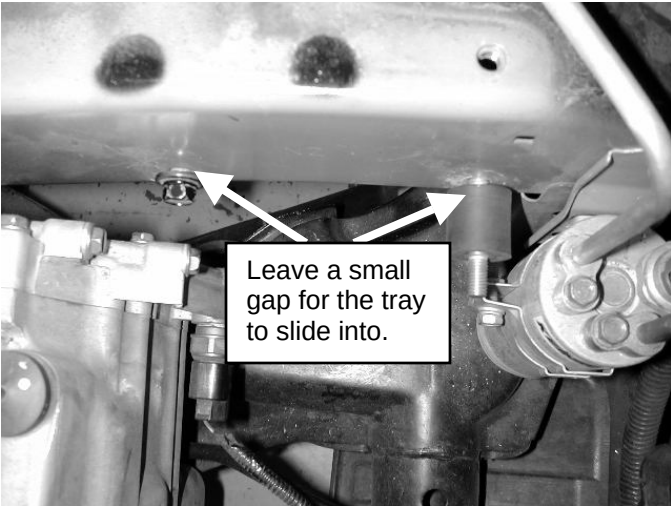
c) Replace the forward of the two lower battery tray bolts with the supplied 1" rubber mount. Do not completely tighten the mount or rear bolt.
