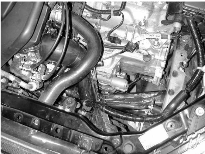
f) Route inlet pipe into the engine bay from the fender towards the throttle body.
