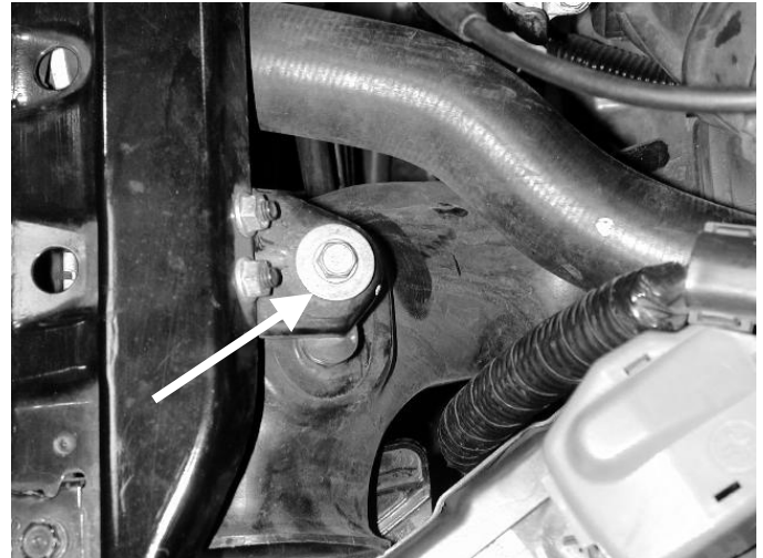
h) Remove the bolt at the air intake snorkel. Remove the stock air box from the vehicle.
