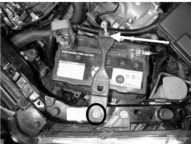
i) Remove the battery hold down bracket. Remove the battery.
