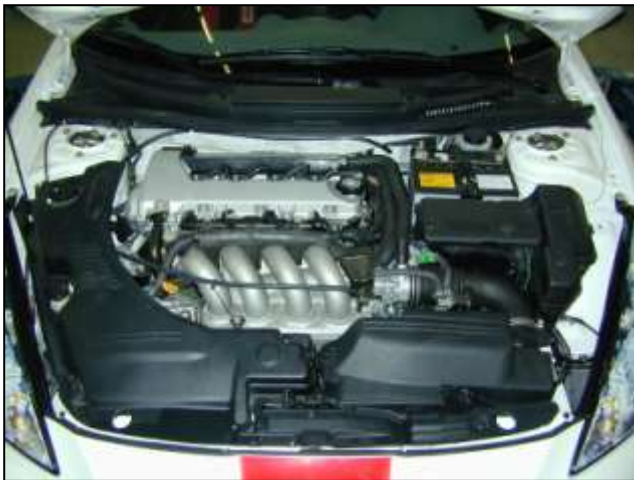
Stock air box system installed
