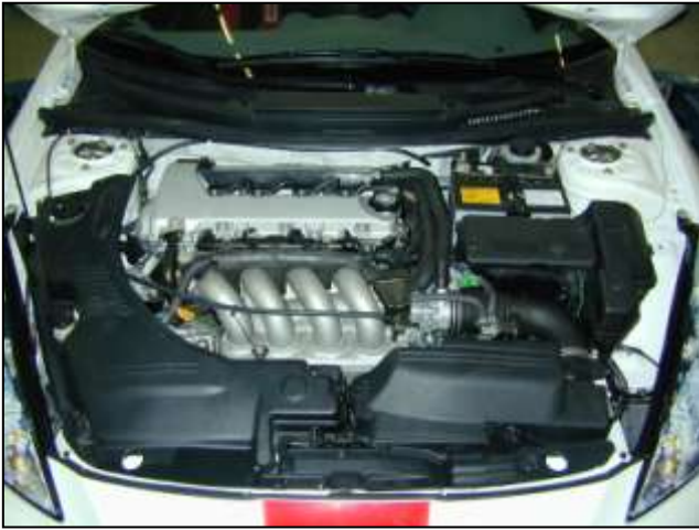
Stock air box system installed
