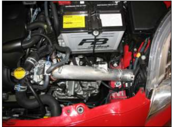
AEM® intake system installed
