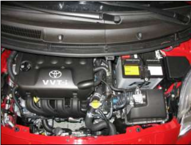
Factory airbox system installed
