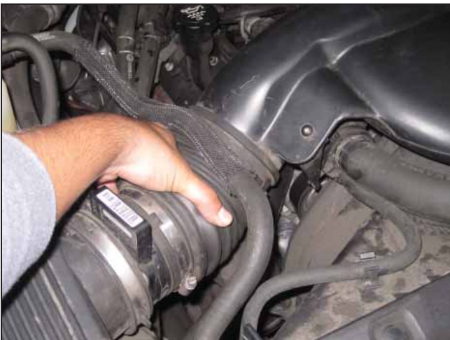
i. Disconnect the intake duct from the MAF sensor.
