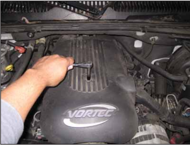
e. Remove the bolt securing the engine cover.
