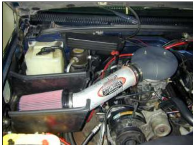
AEM® intake system installed
