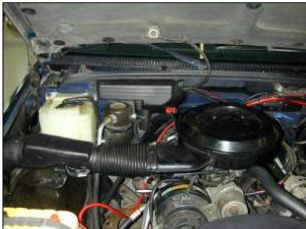
Factory air box system installed
