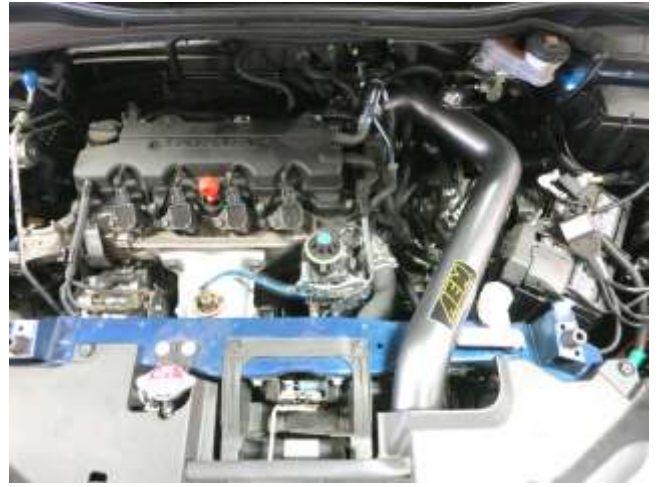
AEM INTAKE INSTALLED
