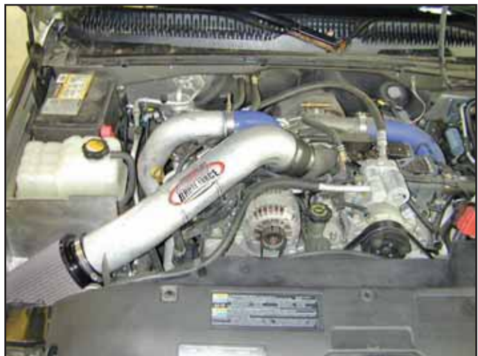
AEM® intake system installed
