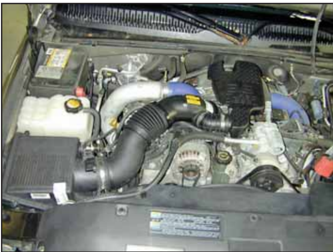
Factory air box system installed
