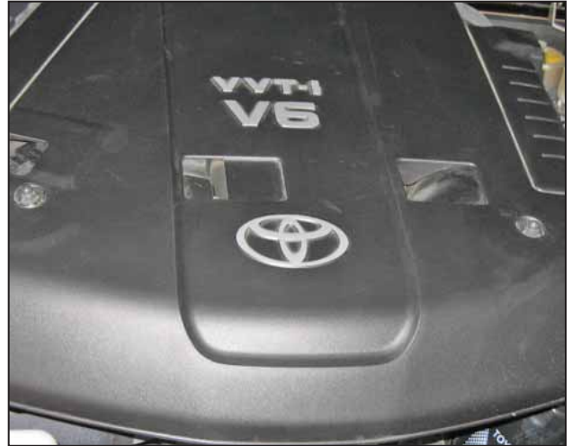
b. Remove the two nuts securing the engine cover.
