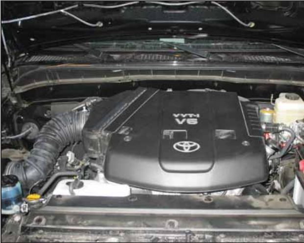
a. Factory airbox system installed.
