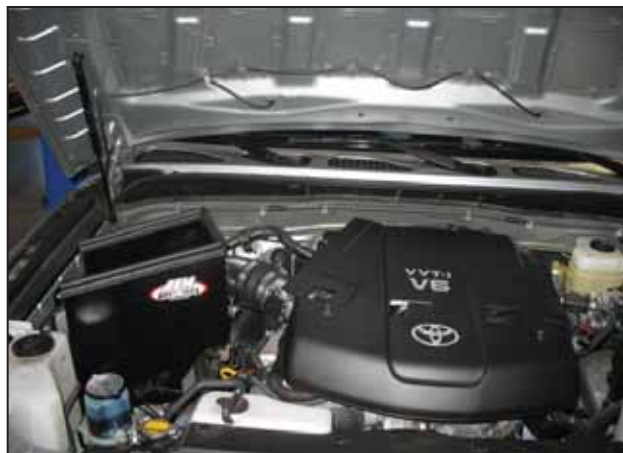
AEM® intake system installed
