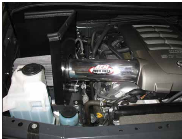
AEM® intake system installed
