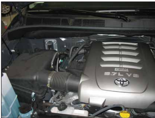
Factory airbox system installed
