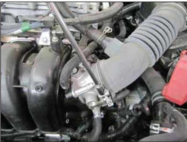
g. Loosen the hose clamp that secures the intake hose to the throttle body.
