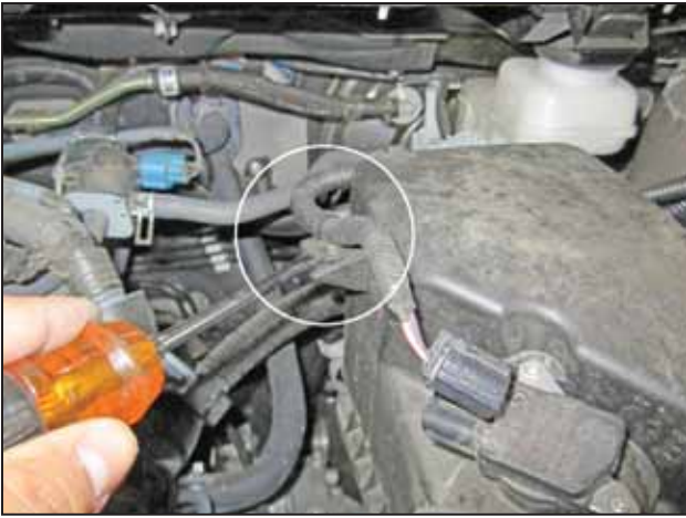
e. Remove the MAF sensor harness clip from the air filter housing.
