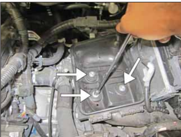
i. Remove the 3 bolts that secure the lower air filter housing to the vehicle chassis.
