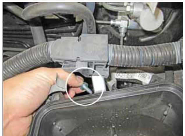
j. Remove the bolt that secures the harness bracket to the back of the lower air filter housing.
