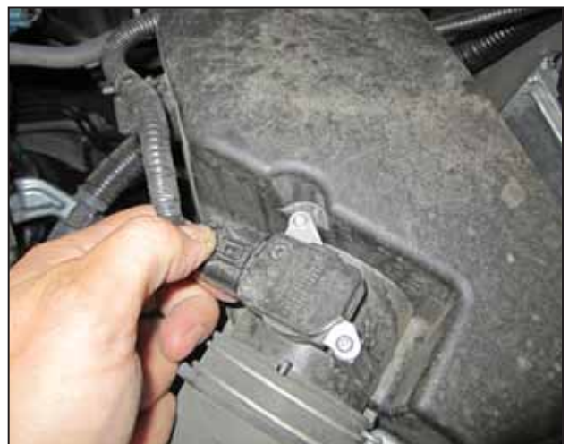
d. Unplug the MAF harness connector from the MAF sensor.
