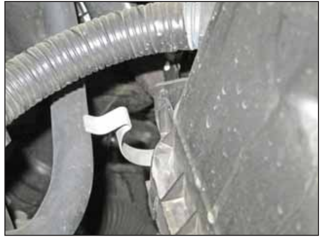
f. Unlock the two clips at the back of the air filter housing.
