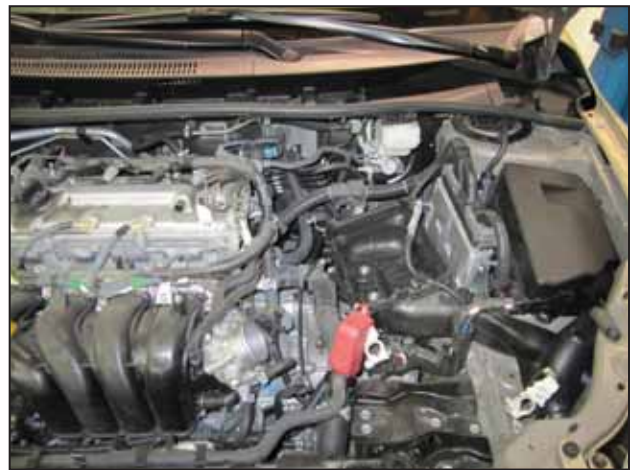
h. Remove the intake hose and upper air filter housing from the vehicle, and then remove the filter element from the lower air filter housing.
