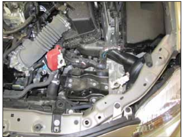
b. Disconnect the positive battery terminal. Remove the battery and plastic battery tray. Refer to the owner's manual for specific details regarding battery removal.
