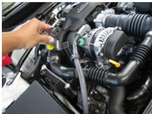
b. Loosen hose clamps on intake sound creator and throttle body. Disconnect plastic tube from sound creator.
