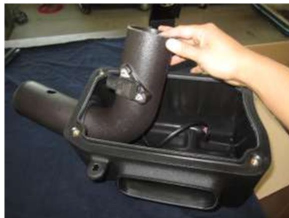
d. Slide intake tube thru the rubber lined outlet from inside of airbox as shown.
