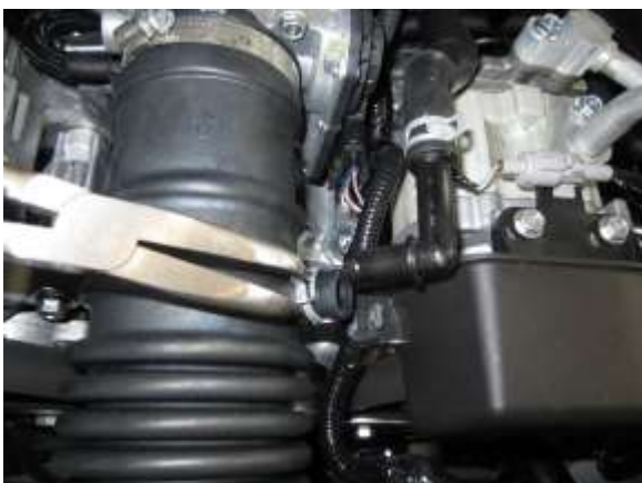
c. Compress spring clamp on rubber intake tube nipple and disconnect plastic elbow from tube. Set spring clamp aside for later use with AEM tube.
