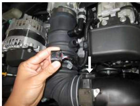
d. Disconnect MAF plug from sensor. Detach gray plastic clip on MAF harness from rear intake box as shown.
