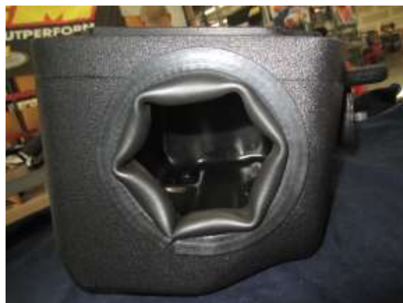
b. Install edge trim(I) along outlet hole of airbox(A) as shown. Trim to fit if necessary.
