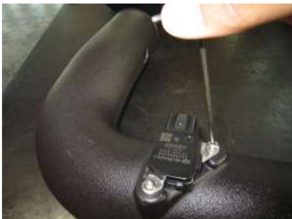
a. Install MAF sensor into intake tube(B) and secure with M4 button screws provided(K).
