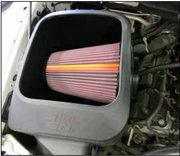
13. Install the K&N air filter into the air filter housing.
