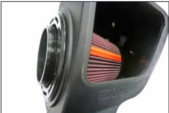
14. Install the air filter into the K&N airbox.
