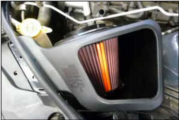
15. Intall the airbox assembly into the vehicle and position to the original airbox mounting studs.
