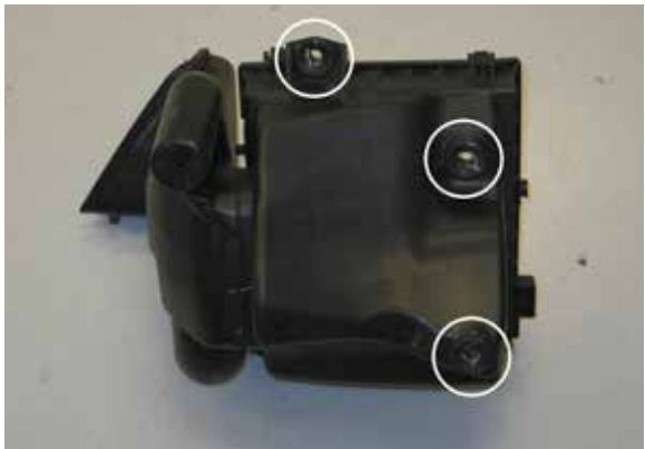
10. Remove three factory airbox mounting grommets from the lower airbox.
