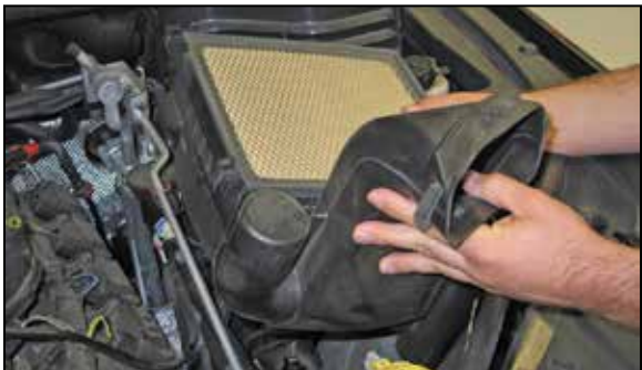
9. Lift up the lower airbox to dislodge it from the mounting grommets and then remove the lower airbox from the vehicle. Some vehicles may have a power steering line attached to the air box than will need to be unhooked. NOTE: K&N Engineering, Inc., recommends that customers do not discard factory air intake.
