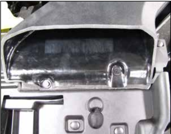
7C. Once the tabs are trimmed flush with the fresh air duct the air filter housing can be installed back into position, pushed down and the locking pins installed as intended.
