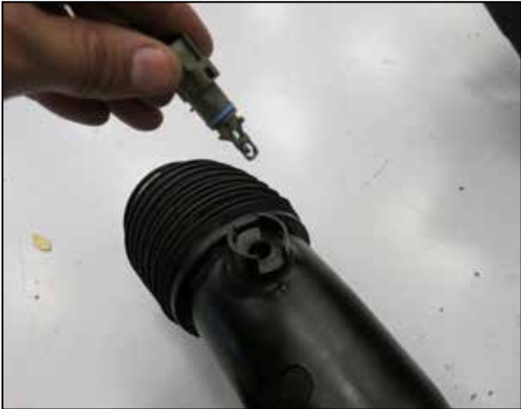
13. Remove the IAT sensor from the factory intake tube.
