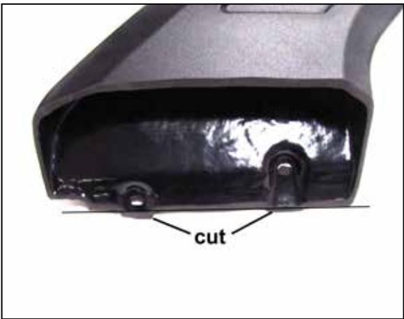
7B. In these cases, it will be necessary to trim the mounting tabs as shown using a hack saw or similar tool.
