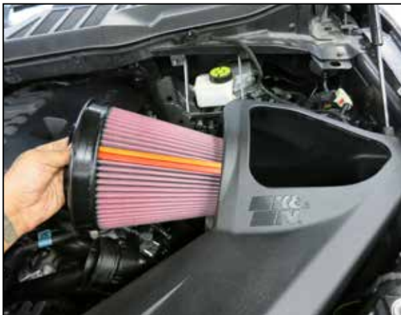
12. Install the K&N air filter into the filter housing.
