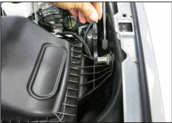
6. Remove the bolt that secures the factory air filter housing to the inner fender and then remove the air filter housing from the vehicle. This bolt will be reused in the next step. NOTE: K&N Engineering, Inc., recommends that customers do not discard factory air intake.
