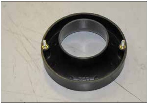
13. Install the two provided 6mm studs into the radius filter adapter as shown. NOTE: Be sure to add a drop of the provided thread locker to each stud before installing into the adapter.
