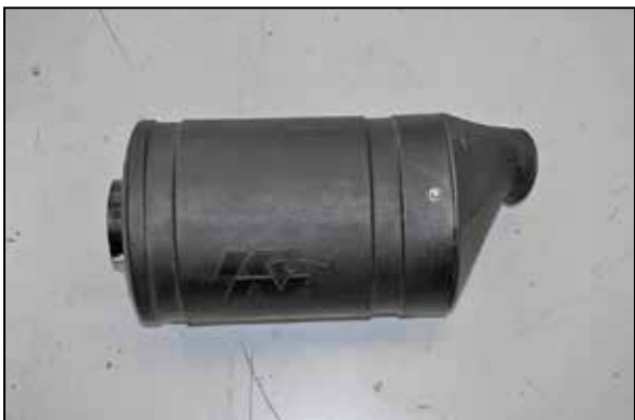
16. Install the end cap into the canister and secure with the provided hardware.
