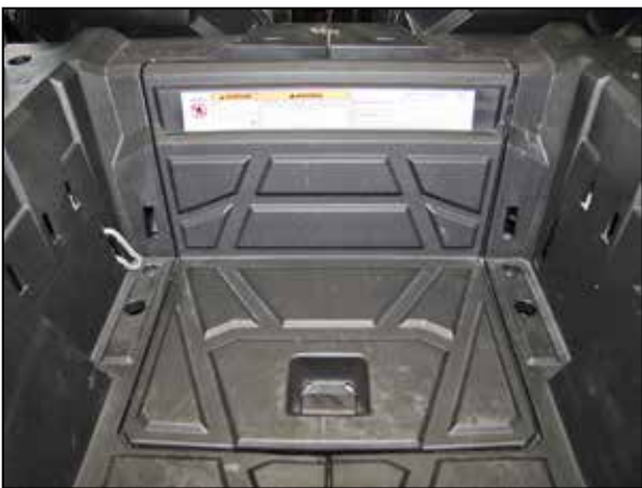
20. Reinstall the factory engine cover.
