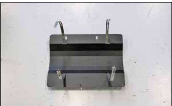
10. Install the two provided large hose clamps through the filter base plate as shown.
