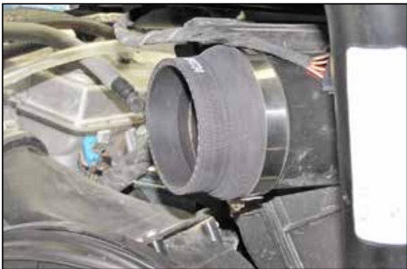
19. Install the provided coupler hose (084034) onto the factory intake plenum and secure with the provided hose clamp.
