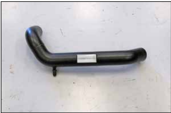
21. Install the provided vent fitting into the K&N® intake tube. NOTE: NPT fitting has tapered threads and only designed to be installed until hand tight, then tighten one rotation or when the fitting becomes difficult to return.
