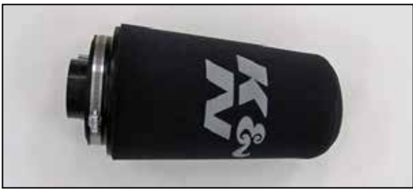
14a. Install the provided foam wrap onto the K&N® air filter.
