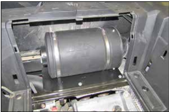
17. Install the filter canister assembly onto the mounting tray and connect the fresh air inlet hose. Adjust the canister and hose for best fit and then secure the canister and hose with the hose clamps. NOTE: Due to differences in the production factory foil heat shield, the heat shield may need to be reformed to allow the canister and fresh air hose to fit together.
