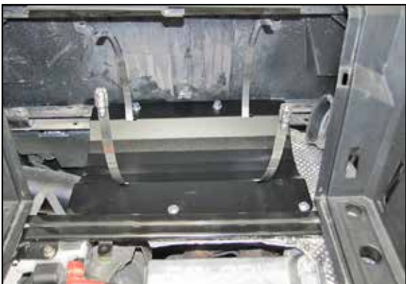
11. Install the filter base plate assembly as shown using the provided hardware.
