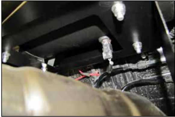
24. Reconnect the inlet air temperature sensor electrical connection.
