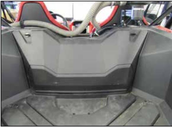
29. Reinstall the air filter access panel and secure with the factory quarter turn fasteners.
