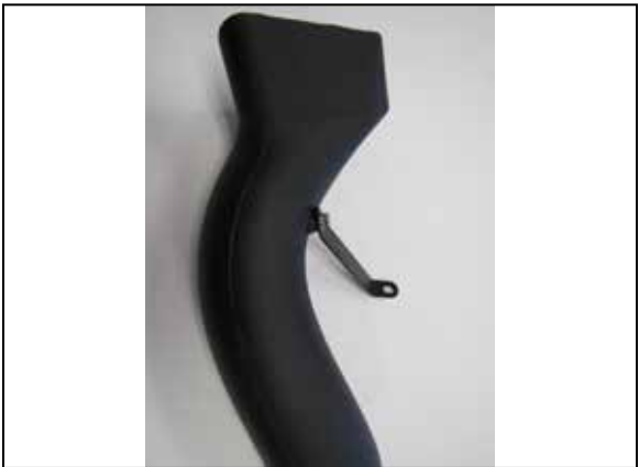
26. Install the fresh air duct mounting bracket onto the K&N fresh air duct using the provided hardware.
