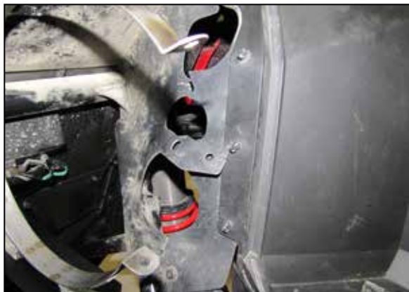
22. Remove the retaining clips and then remove the fresh air duct seal.
