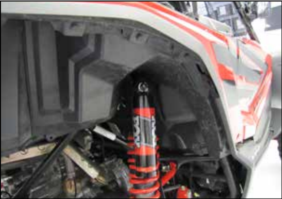
28. Reinstall the fresh air intake duct cover and the original mounting clips.
