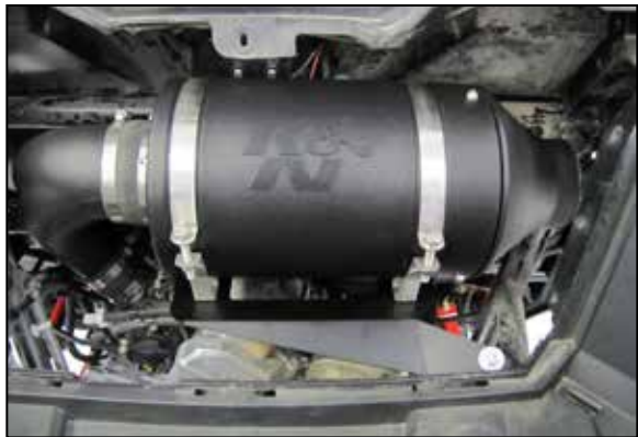
23. Install the K&N air filter assembly along with the provided large hump coupler. Secure the housing with the clamps and secure the coupler with the hose clamps.
