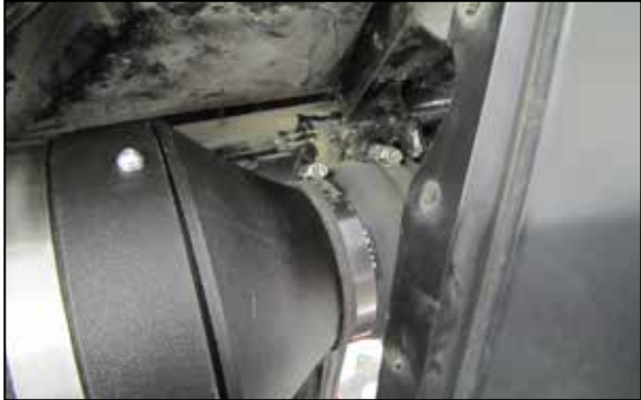
25. Install the smaller hump coupler onto the filter housing inlet and secure with the provided hose clamp.
