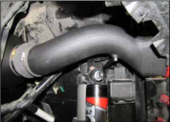
27. Install the fresh air duct into the coupler and then align the bracket, adjust the duct for best fit and then secure with the provided hardware and hose clamps.
