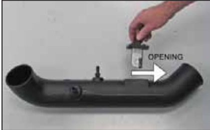
21. Install the mass air sensor assembly into the K&N® intake tube and secure with the provided hardware. NOTE: Be sure to install the mass air sensor in the correct direction, the opening is to be towards the filter end of the tube.
