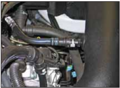
23. Connect the crankcase vent hose to the quick disconnect fitting in the K&N® intake tube.
