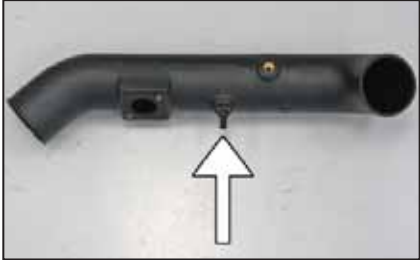
16. Install the provided 3/8" hose fitting into the K&N® intake tube as shown.
