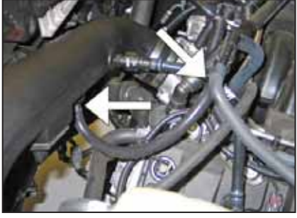
24. Install the provided silicone hose onto the 3/8" fitting installed in the K&N® intake tube and then attach the open end to the EVAP check valve.
