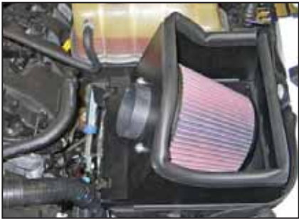
13. Install the heat shield/filter assembly onto the lower airbox and secure with the factory airbox retaining clips. NOTE: A gap is normal between the lower airbox and the heat shield on the clip side of the heat shield.
