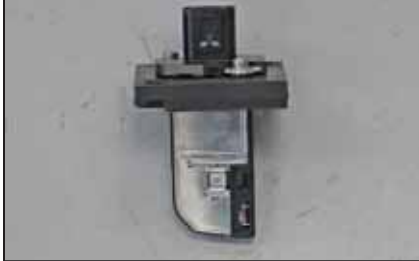
20. Install the mass air sensor into the K&N® sensor adapter as shown. Secure with the provided hardware.
