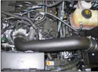
22. Install the K&N® intake tube assembly into the silicone hose at the filter adapter and then into the silicone hose on the throttle body and secure with the provided hose clamps.
