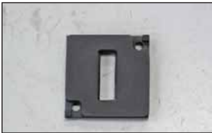
18. Install the provided gasket onto the mass air sensor adapter as shown.
