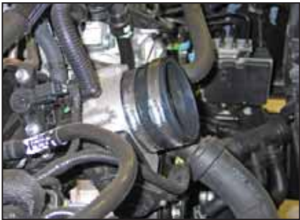
14. Install the provided silicone hose (08630) onto the throttle body and secure with the provided hose clamp.
