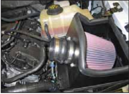
15. Install the provided silicone hose (084057) onto the filter adapter and secure with the provided hose clamp.
