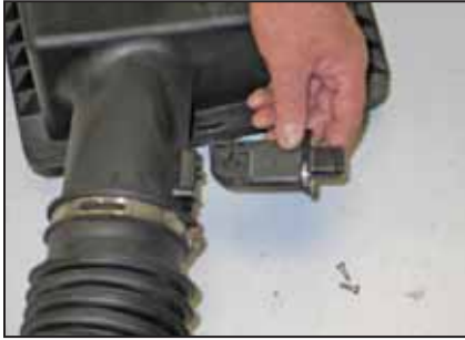
19. Remove the two screws securing the mass air sensor and then remove the mass air sensor from the stock intake tube as shown.
