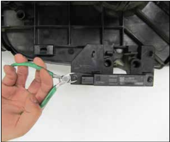
21. Peel the backing off the heat barrier and then apply the barrier to the engine side of the heat shield as shown. After the heat barrier is installed, use a knife or similar tool to cut out all of the mounting holes in the heat shield through the heat barrier.
