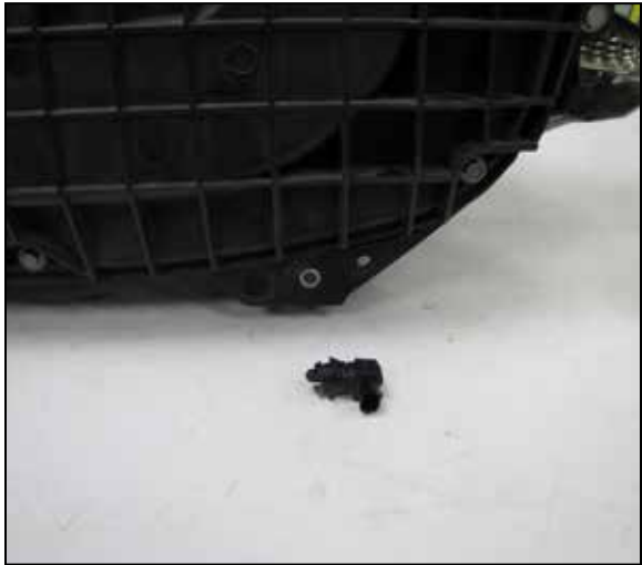
23. Remove the air temperature sensor from the air filter housing.
