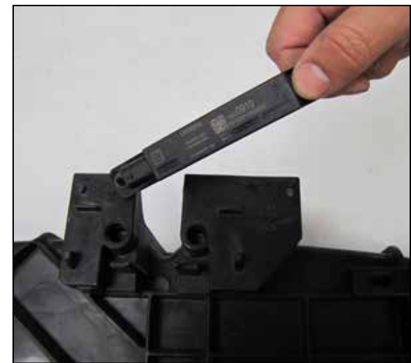
22. Cut the sonic welds that secure the “F” antenna to the air filter housing and then remove the antenna from the housing.
