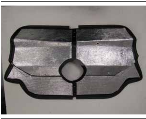
21. Peel the backing off the heat barrier and then apply the barrier to the engine side of the heat shield as shown. After the heat barrier is installed, use a knife or similar tool to cut out all of the mounting holes in the heat shield through the heat barrier.
