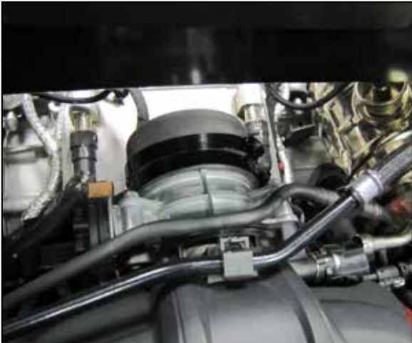
18. Install the coupler onto the throttle body and secure with the provided hose clamp.
