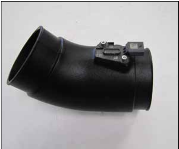
26. Remove the mass air sensor from the factory air filter housing and install it into the K&N intake tube using the provided hardware.
