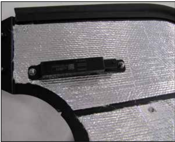
24. Install the “F” antenna to the engine side of the driver’s side heat shield assembly using the provided hardware with the button head of the bolt on the filter side of the heat shield.
