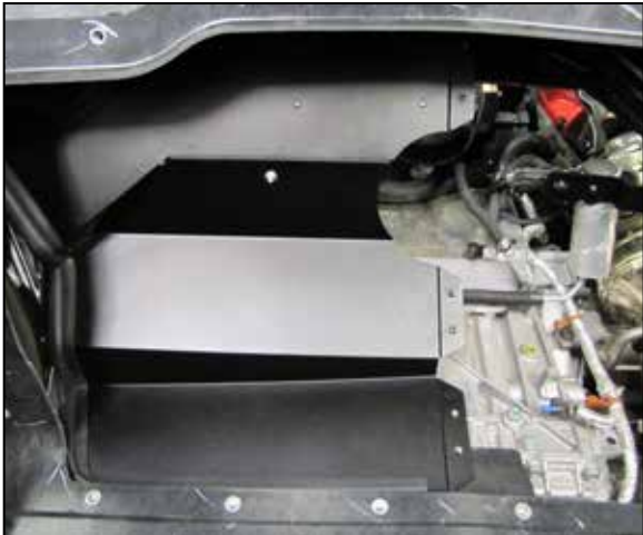
25. Install the drivers side heat shield assembly and align with the mounting bracket. Secure the heat shield with the provided hardware. Reconnect the “F” antenna electrical connection.
