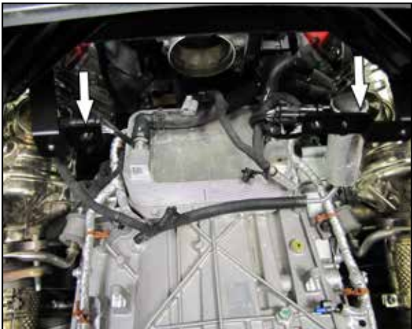
17. Attach the transmission vent reservoir and o2 wiring harness to the heat shield mounting brackets.
