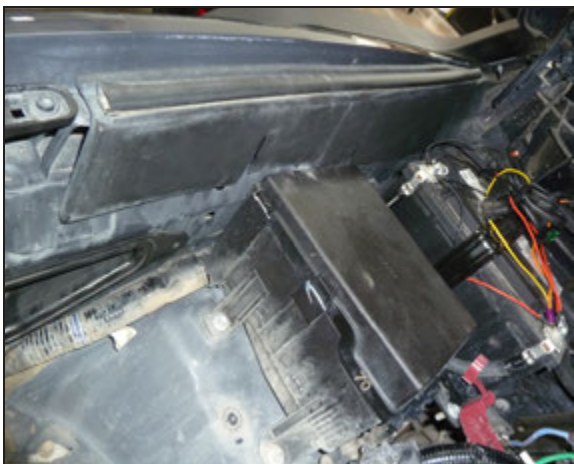
25. Re-install the under-hood plastic fender liner.
