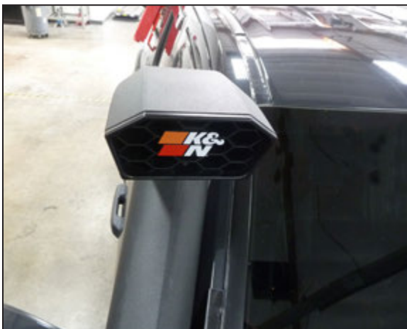
27. Install the snorkel top onto the snorkel and secure with the provided hose clamp.
