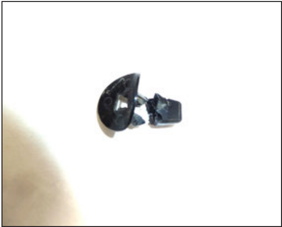
5. Gently pull the inner fender liner down to access the inside of the fender. It will be necessary to cut the plastic clips nuts to lower the fender liner, replacement clip nuts are provided.
