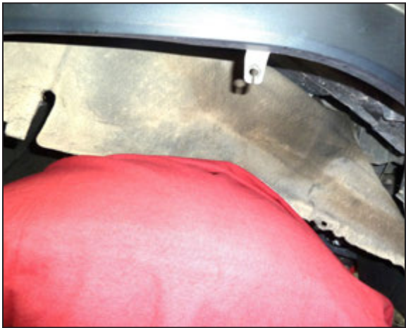
7. Place the template onto the fender aligning it with the top edge of the fender as shown. NOTE: Double check the alignment before going to the next step.
