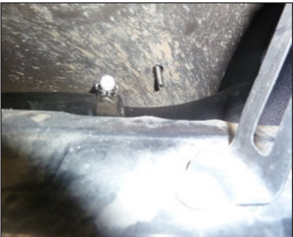
22. Install the remaining stud into the front insert of the snorkel.
