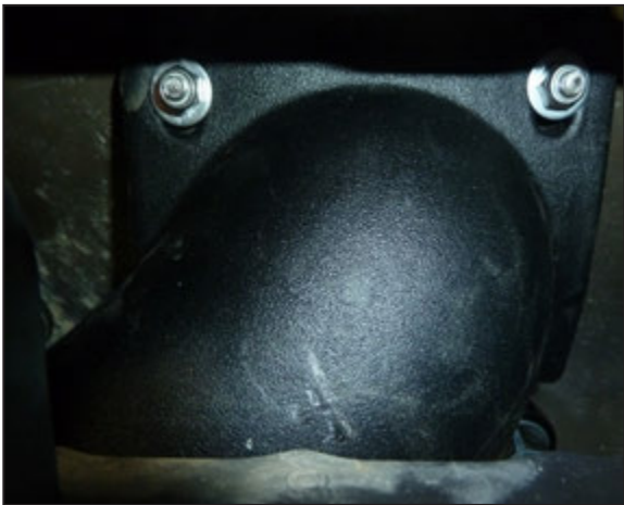
23. Install the four smaller washers and nylock nuts onto the studs to secure the inner fresh air tube to the snorkel but do not tighten. The lower front nut and washer will be a challenge due to the tube, take your time and be patient.
