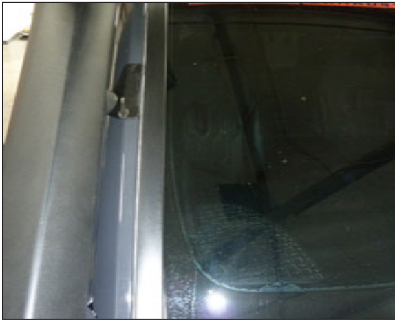
26. Reinstall the passenger side windshield trim.
