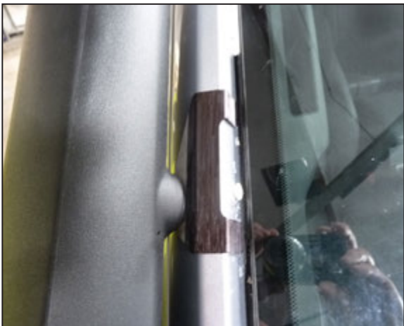
21. Peel the remaining double-sided tape backing off and then install the snorkel assembly onto the fender so that the mounting studs pass through the mounting holes and the mounting bracket is around the A-pillar.
