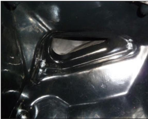
29. Re-install the K&N air filter housing and secure it to the inner fender with the provided bolts. The bolts will pass through the air filter housing and the fresh air duct into the threaded holes in the inner fender. Reassemble the intake system.
