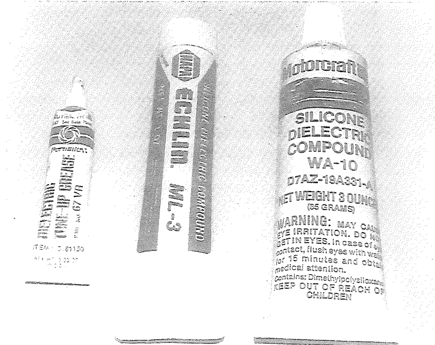
Figure 7.8. Some of the safe lubricants you can use in place of the Dow-Corning 111 grease. Oddball lubricants may damage rubber brake parts.
