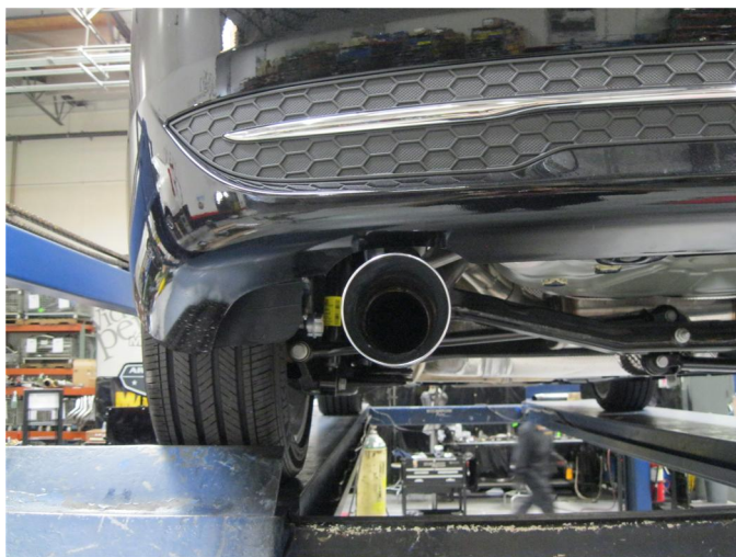
Step 6. Once a final position has been chosen for the new exhaust system, evenly tighten all clamps from front to rear using the torque specifications on page one of the instructions. Inspect all fasteners after 25-50 miles of operation and re-tighten if necessary.
