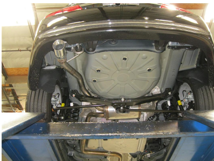
Step 5. Tail Pipe Assembly installed.
