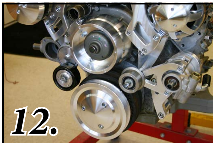
Photo 9: Apply Loc-Tite to the threads of the three \frac{3}{8} "-16 x 1" SHCS (S248) and install Crank Pulley to the March Crank Adapter Hub
