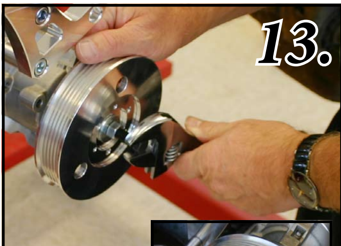
Photo 13: Press power steering pulley (619-A) on with an install tool or bolt and washer as shown. When properly installed pulley should be flush with top of shaft as shown.
