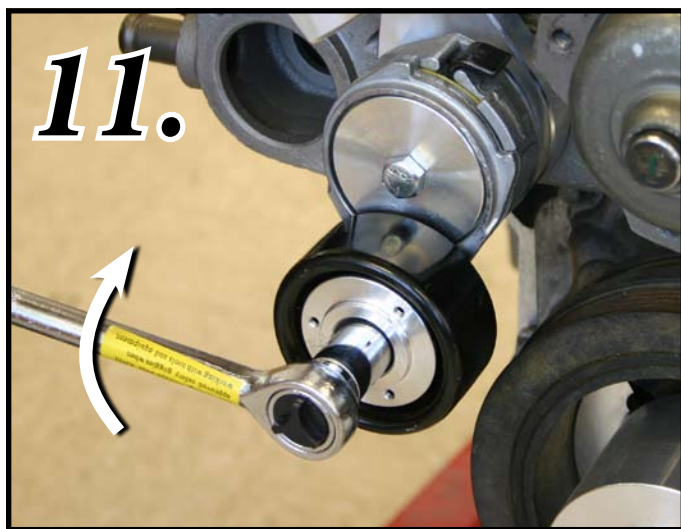
Photo 11: Temporarily mount the OEM style tensioner (P756) to Tensioner Base (20069-A) using one \frac{3}{8} "-16 x 2 \frac{1}{4} " Hex Head Bolt (S324) , Be sure to align pin on rear of tensioner with hole in tensioner base. This will aid you in removing the tensioner pulley. Remove the pulley bolt using a 15mm wrench and discard the washer.
