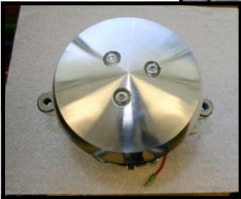
Photo-9 Install the alternator fans (221-A) and the two Alternator pulleys (208-A) to the two Alternators.(P572) then install the two Alternator Caps (307-A)
