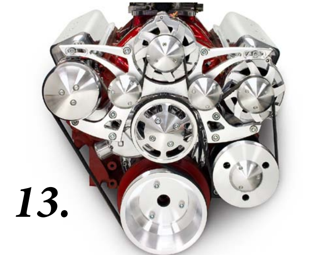
FIG 14. Pull the Alternator and A/C units outward to take up slack in the belt and center both units at the top adjustment slot. Tighten either the A/C or Alternator 8mm top adjustment slot bolt and using an apropearte pry bar pull the other unit outward to achieve proper belt tension, Tighten the top mounting bolt on that unit.
