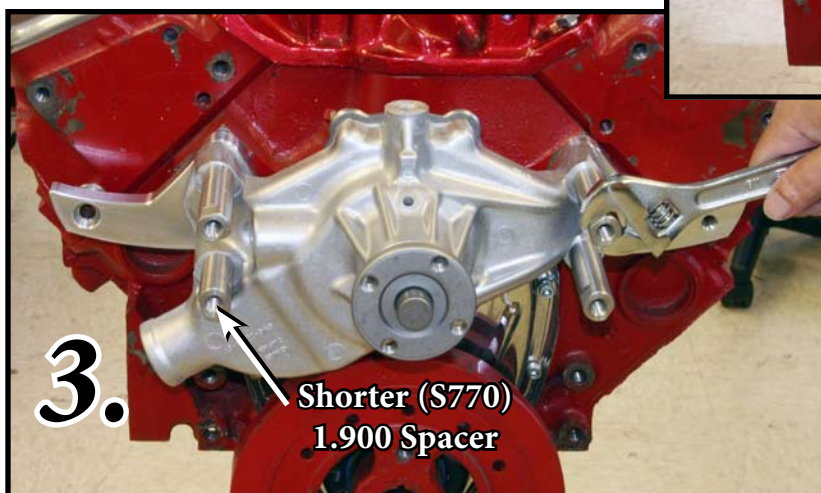
FIG 3. Slide the Water Pump (P112) Over the Studs and secure with the (3) \frac{3}{8} x 2.800" Stainless Spacers (S775) two to the upper water pump studs and one to the lower drivers side water pump stud. Install (1) \frac{3}{8} x 1.900" Stainless spacer (S770) on to the lower passenger side water pump stud. Use a sealer if nessessary.
