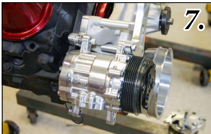
Fig 7. Install A/C unit (P412) Using a M8 x 20mm SHCS (S550) in the lower front hole and a \frac{5}{16} x 1\frac{1}{2} " (S150) SHCS in the rear lower Hole. Use a \frac{3}{8} " I.D. x .300 long spacer (TP3-.300) between the rear A/C bracket and the rear ear of the A/C unit As Shown.
