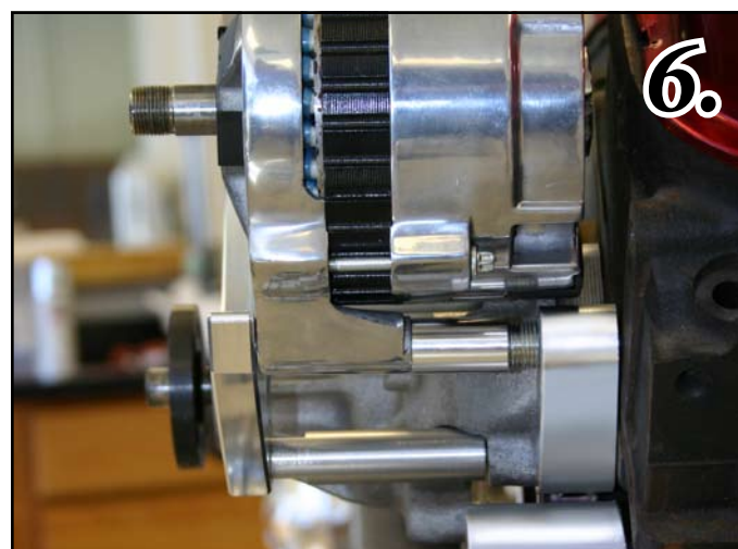
Fig 7. Install A/C unit (P412) Using a M8 x 20mm SHCS (S550) in the lower front hole and a \frac{5}{16} x 1\frac{1}{2} " (S150) SHCS in the rear lower Hole. Use a \frac{3}{8} " I.D. x .300 long spacer (TP3-.300) between the rear A/C bracket and the rear ear of the A/C unit As Shown.
